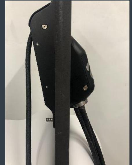
Fit halyard and check operation of the lock
